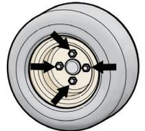
8. Fully remove the (8) rear lug nuts, tires and wheels. Discard.
