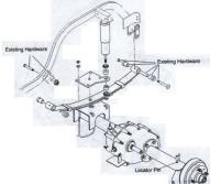
new shock mounting plate on top of spring. Install rear leaf spring shackle with existing hardware. Tighten hardware. Install and tighten the front spring existing hardware.
