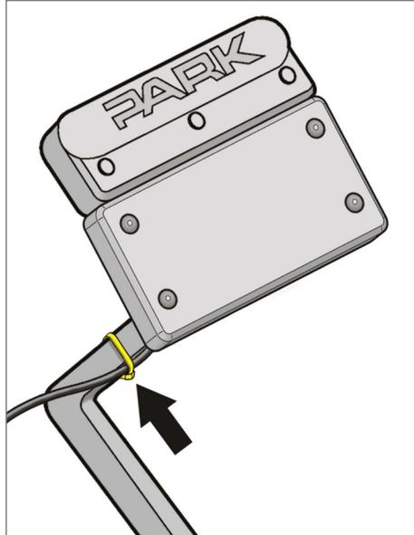
8. Connect the LGT-B10 to the RHOX plug & play wire harness per the light kit's instructions.
