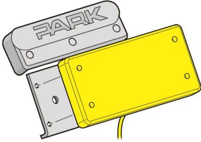
5. Attach the LGT-B10 to the brake pedal plate with the (4) Included Rivets.
