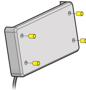
4. Place the LGT-B10 over the brake pedal plate with the wire at the bottom.
