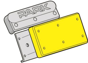
3. Push Spacers in the (4) holes of the new LGT-B10 brake pad.
