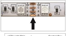
6. Connect the LED strip to the wireless controller at the 4-pin connector.
